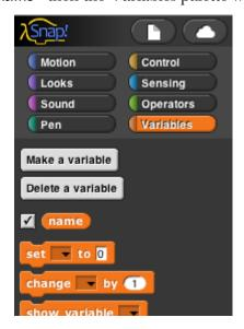
There's now a "**Delete a variable**" button, and there's an orange oval with the variable name in it, just like the orange oval in the **for** block. You can drag the variable into any script in the scripting area. Next to the oval is a checkbox, initially checked. When it's checked, you'll also see a *variable watcher* on the stage:
