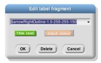
This says to make the symbol **1.5** times as big as the letters in the block text, using a color with red-green-blue values of **255-255-150** (each between 0 and 255). Here's the result:
