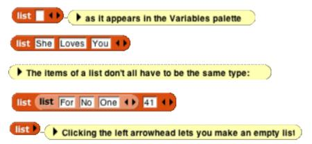
At the right end of the block are two left-and-right arrowheads. Clicking on these changes the number of inputs to **list**, i.e., the number of elements in the list you are building.
